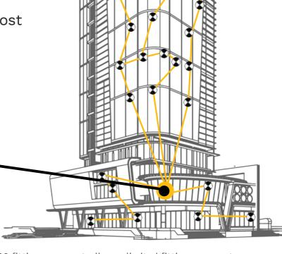
\*1000 fittings per controller, unlimited fittings per system. Location of the controller is flexible & can be moved should the need arise.
