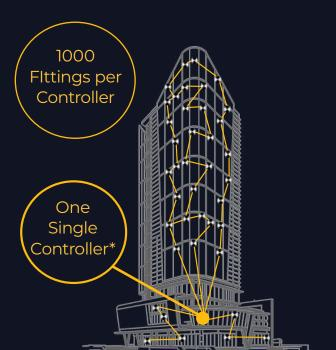
\*1000 fittings per controller, unlimited fittings per system. Location of the controller is flexible & can be moved should the need arise
